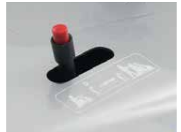
This unique two-step disengaging lever prevents the scooter from accidentally freewheeling.
